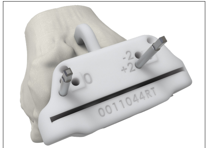
Figure 15. F2 placed onto previously created pin-holes
