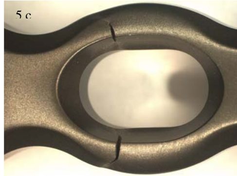
Figure 5: Screw-pull-out – a) Failure of plate, b+c) detailed view of failed plate, b) Stryker® XXL Volar DR VariAx Plate, c) Stryker® SPS plate
