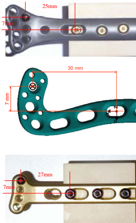
Figure 2: Lever arms of the different test setups (Upper: Stryker® XXL Volar DR VariAx Plate, Middle: Zimmer® Distal Volar Radial Radius Plate, Lower: Synthes® LCP Dia-Meta Volar Distal Radius Plate)
