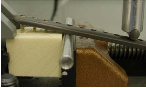
Figure 4: Screw-pull-out - Failure of construct with Stryker® 3x2.7mm VariAx DR Bone screws in poor quality bone model (10pcf PU-foam)
