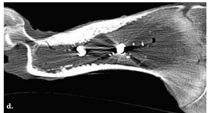
Effect of peak voltage on metal-related artifacts. A comparison of CT images obtained through the short axis of the screws in the pig femur model, with 140 kVp **(c)** and 80 kVp **(d)** and with other parameters the same (120 mAs, 0.6-mm collimation, and 1.0-mm reconstructed section thickness), shows a less obtrusive artifact on the image obtained with a higher peak voltage.<sup>18</sup>
