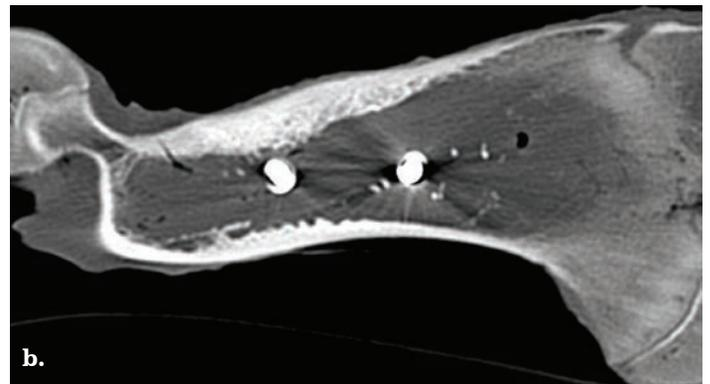
Effect of metal composition on metal-related artifacts at multidetector CT. **(a)** Scout view of an ex vivo model of a pig femur with a 4.5-mm titanium alloy screw (arrow) and a 4.5-mm stainless steel screw (arrowhead). **(b)** CT image obtained through the short axis of the screws, with 140 kVp, 120 mAs, 0.6-mm collimation, and 1.0-mm reconstructed section thickness, shows more severe streak artifacts from the stainless steel screw than from the titanium alloy screw.<sup>18</sup>
