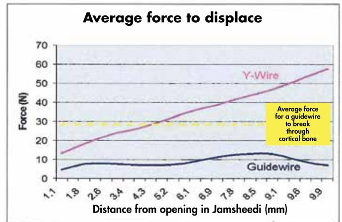
Figure 2. Average force for a guidewire to break through cortical Bone
