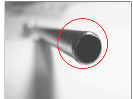
Tissue protection sleeve: dents on the sleeve tip
