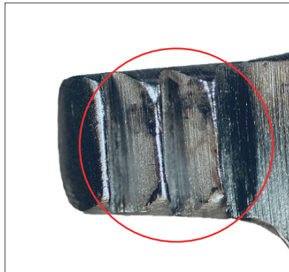
Bent teeth and damaged locking mechanism on a forceps
