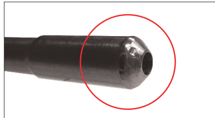
Drill guide sleeve: dents on the sleeve tip
