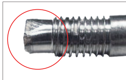
Connection rod of Gamma lag screwdriver: damaged and squeezed thread
