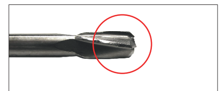
Blunt / dull tip Please check at tip of drill (see mark)
