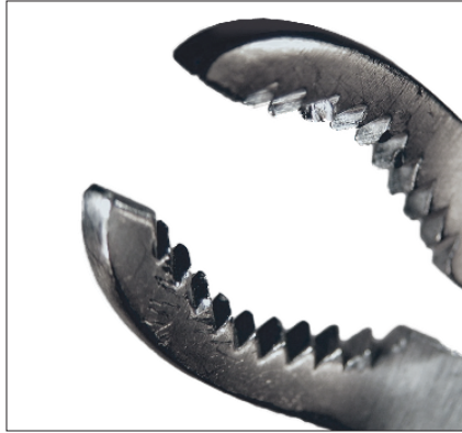
Bent teeth and damaged locking mechanism on a forceps
